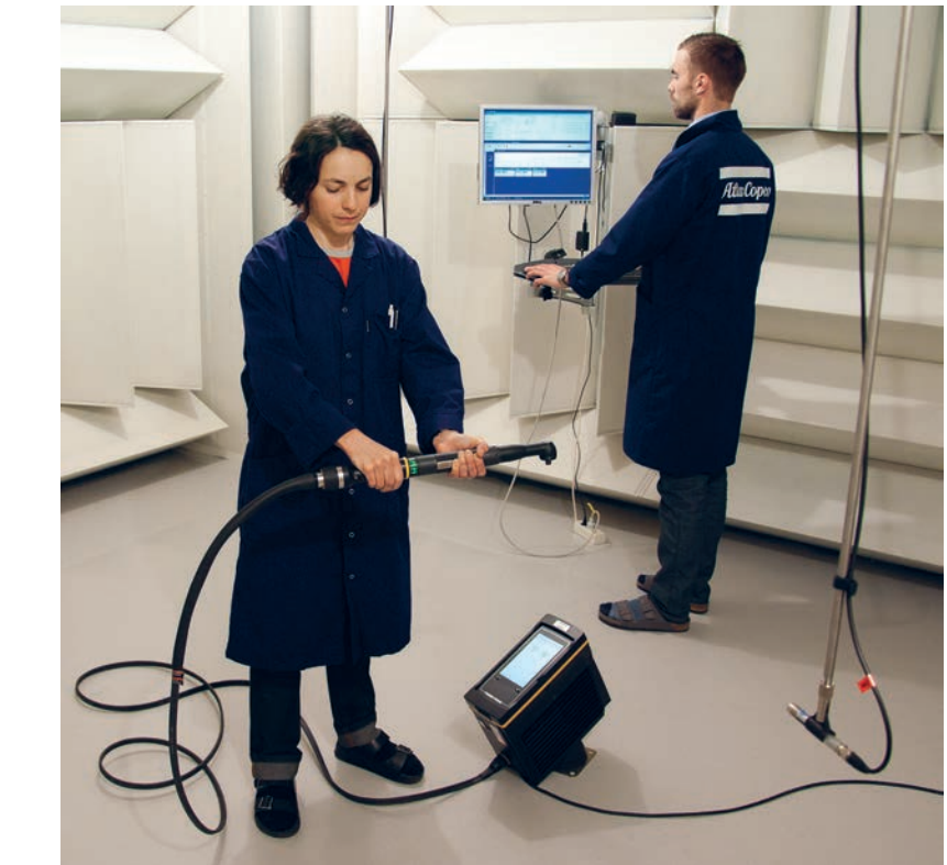
Atlas Copco has a well equipped laboratory for measuring tool noise and vibration emissions. It contains advanced vibration measurement tools, a state-of-the-art acoustics laboratory and dedicated computer software for analysing measurement and test results.
